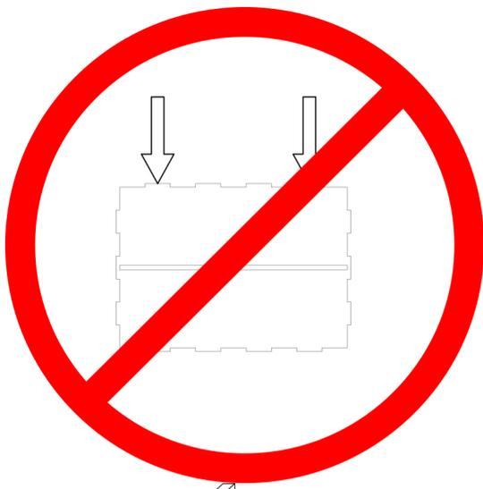
Never put pressure on the part with long slot perpendicular to the slot. It will snap. Always start assembly with the shorter, side, pieces. This will strengthen the part and stop it from snapping when pressure is applied. If it does snap it is still possible to put it together but it makes it harder.
