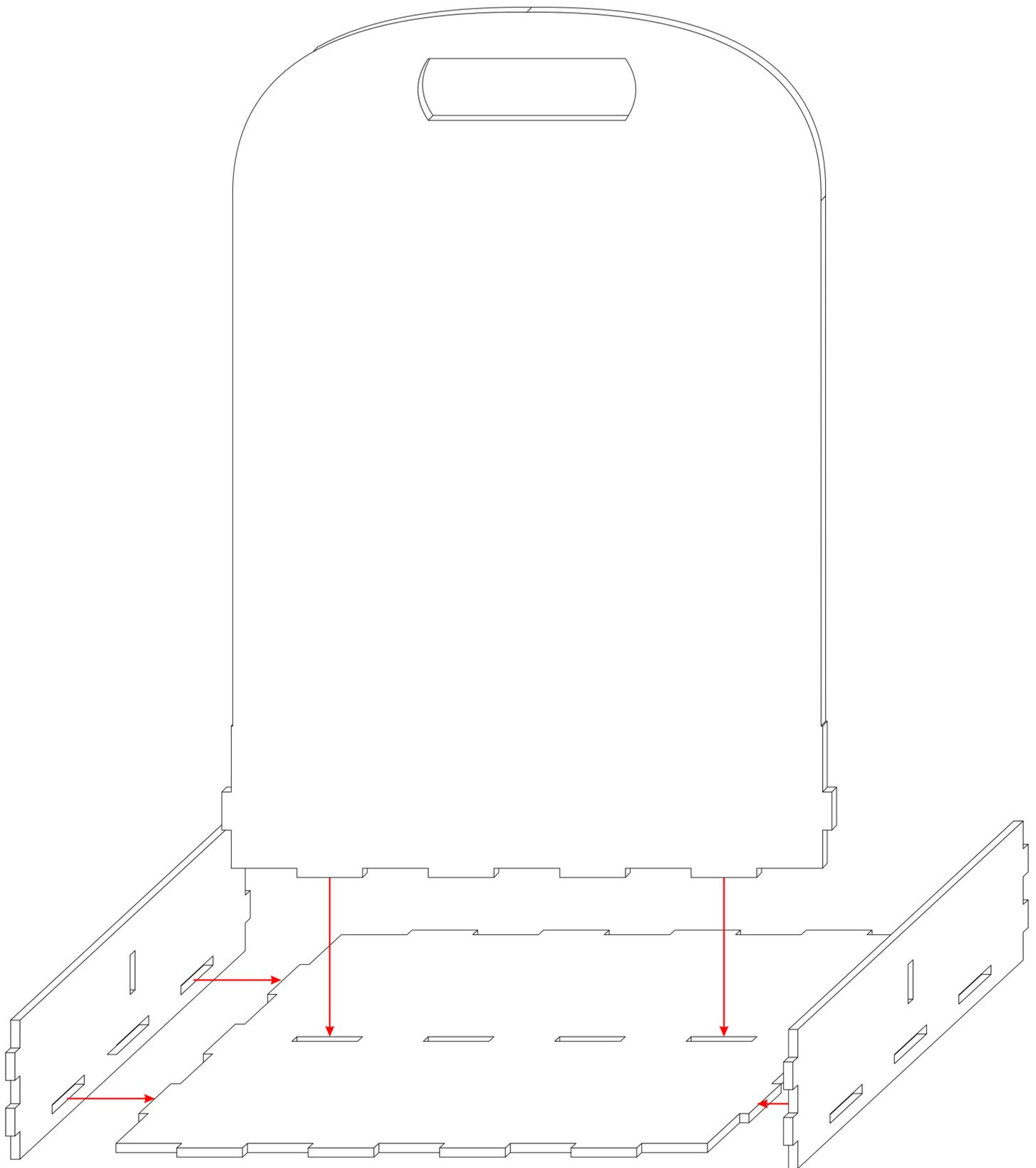
Start the bottom tray by gluing the divider/handle part first. Follow with the side elements. Clamp and leave to dry.
