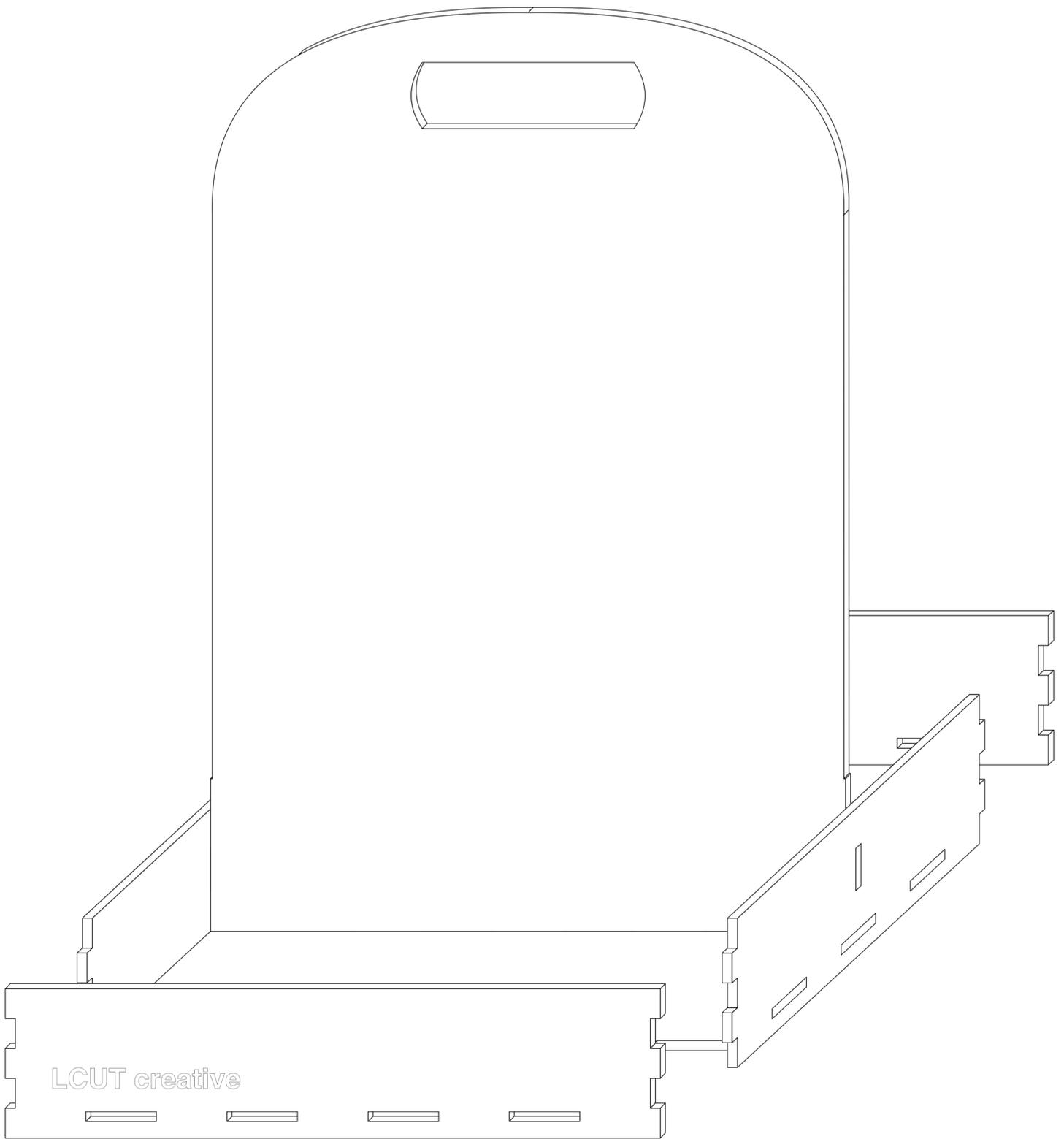
Finish off the bottom try by gluing the longer, front and back elements. Clamp and leave to dry.
