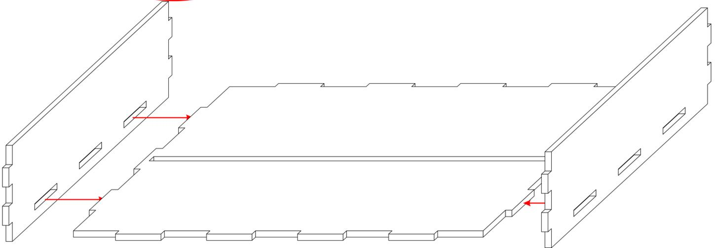
Start assembly of removable tray by gluing the shorter sides first. Clamp and leave to dry. The slots may be tight fitting, use file/sand paper to clean them up and ease assembly. Use plenty of wood glue.
